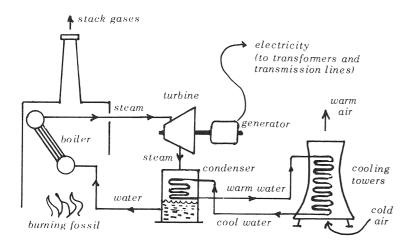
How a power plant works. Schematic drawing showing the barest principles, omitting economizers, superheaters, reheaters, feedwater heaters, high and low pressure turbines, pumps and other elements.
